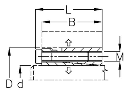
B mm = 60d H8 mm = 75D mm = 115Fit tolerance = Aksel h8, Nav H8F kN torque = 210L mm = 70M mm = 100P N/mm2 surface pressure on shaft/hub = 130
